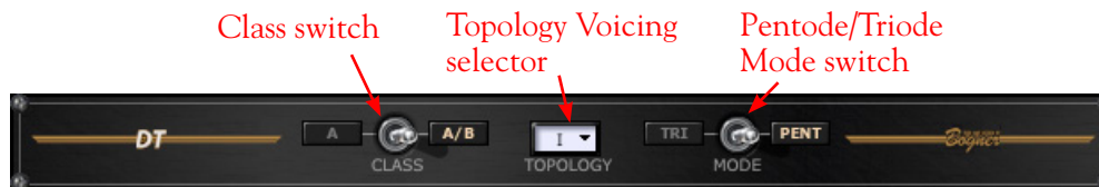
Amp Panel - DT50 amp controls
